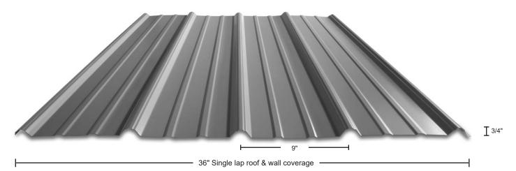
Ultra-Panel's positive side lap keeps panels square and acts as an excellent anti-siphon that prevents leakage at the seams - eliminating the need for side lap tape and stitch screws. Because the side lap is virtually invisible, the Ultra-Panel has a clean, attractive appearance.
