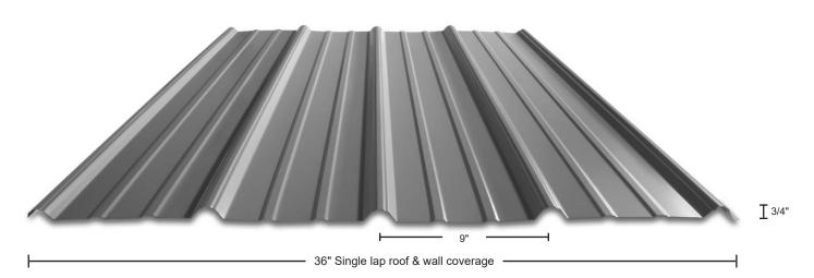
Ultra-Panel's positive side lap keeps panels square and acts as an excellent anti-siphon that prevents leakage at the seams - eliminating the need for side lap tape and stitch screws. Because the side lap is virtually invisible, the Ultra-Panel has a clean, attractive appearance.
