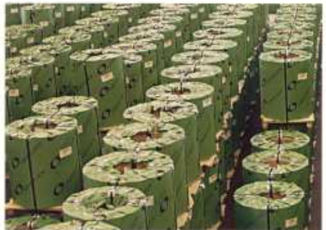
Double stacked, vertical skidded coils properly stored in a controlled environment.
